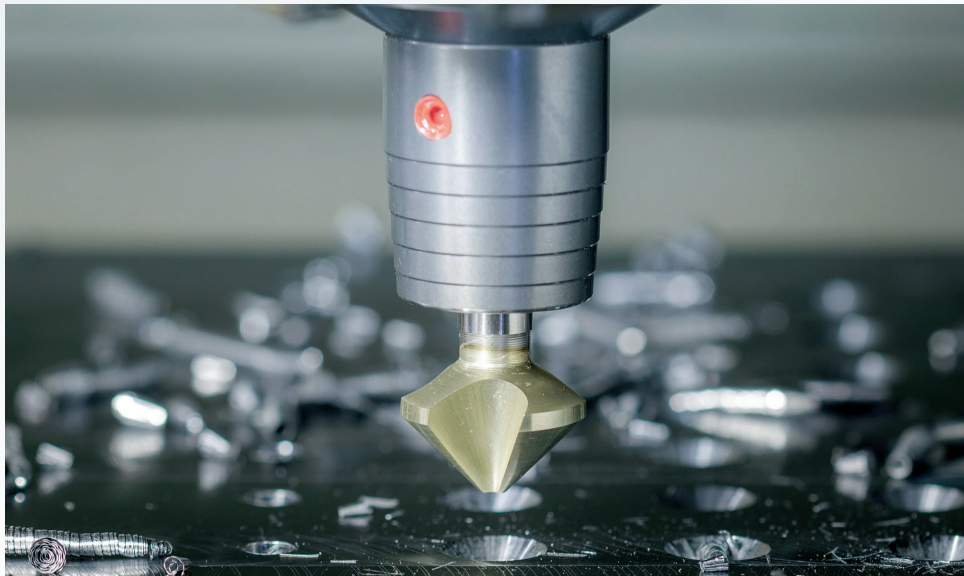
Standard-Senker 42CrMo, v_c = 15 \text{ m/min} , f_u = 0.15
