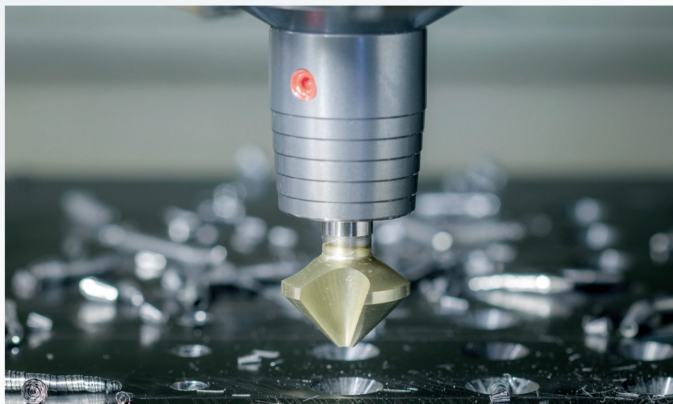
Standard-Senker 42CrMo, v_c = 15 \text{ m/min} , f_u = 0.15
